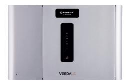
The NOTIFIER Intelligent VESDA-E SLC with VESDAnet detectors (referred to as 2<sup>nd</sup> gen. detectors) have an integrated Signaling Line Circuit (SLC) module to communicate with NOTIFIER Fire Alarm Control Panels (FACP) directly over the SLC loop. The 2<sup>nd</sup> gen. detectors are variants of the conventional VESDA-E detectors with built-in SLC interface module.
